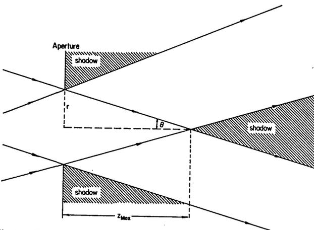
Fig. 6. Geometrical shadow zone for  $J_0$  beams of finite aperture. A conical shadow zone begins at the distance  $z = r/\tan \theta$ , where  $r$  is the radius of the limiting aperture at  $z = 0$ ,  $\theta = \sin^{-1}(\alpha\lambda/2\pi)$ , and the diameter of the central maximum of the  $J_0$  beam is approximately  $3\pi/2\alpha$ .
