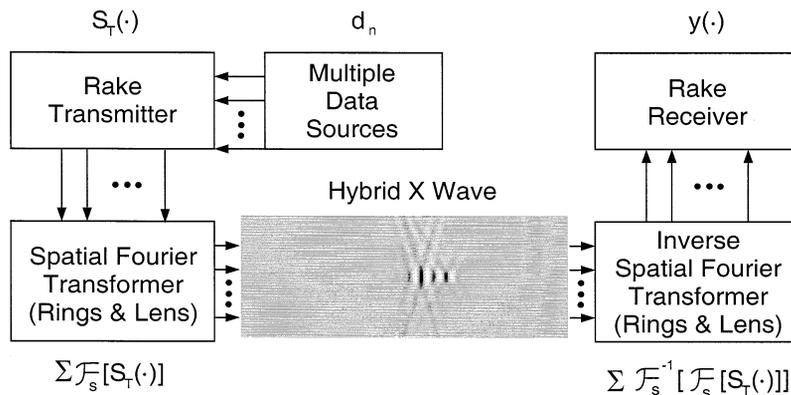
Fig. 1. Model of the optical X wave communication systems.
