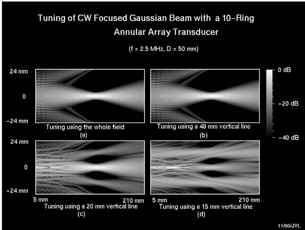
Fig. 10. Tuning results for a CW focused Gaussian beam. (a) Tuning result using the whole field Fig. 9(a). (b) Tuning result using a 48-mm vertical line of the field in Fig. 9(a) through the focal distance  $z = F = 120$  mm. (c) Same as (b) but with vertical line of 20 mm. (d) Same as (b) but with vertical line of 15 mm.
