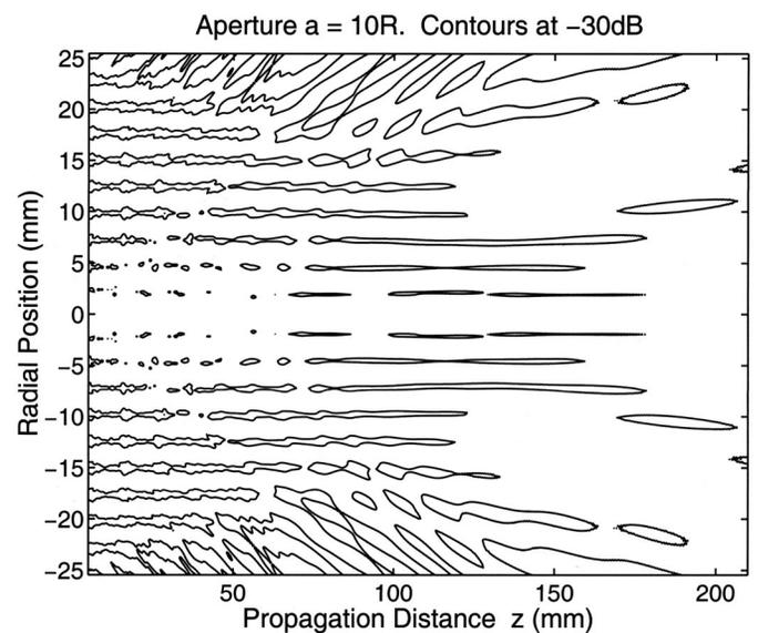
Fig. 5. -30 dB contour levels for field calculation with  $a = 10R$ .
