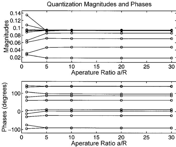
Fig. 12. Convergence of quantization magnitudes  $|q_p|$  and phases  $\theta_p$  as a function of aperture ratio  $a/R$  for tuning example in Fig. 11(b).
