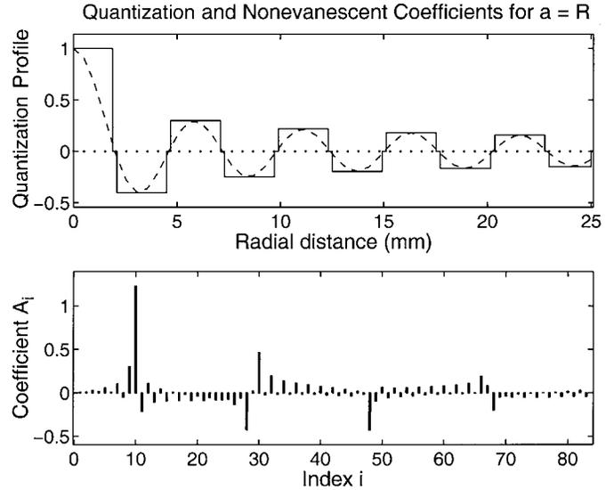
Fig. 1. Quantization profile (upper) and nonevanescient Fourier-Bessel coefficients  $A_i$  (lower) for modelling aperture  $a = R$ .
