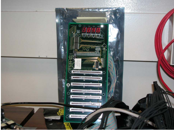
Figure 6. Front panel board. The board has a 4-digit LED display for system messages. It contains 8 TGC sliders and passes the signals from the buttons on the front panel to the main board.
