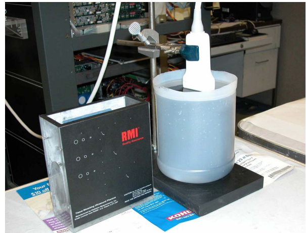
Figure 9. Experiment setup for data acquisition using the high frame rate imaging system. A standard RMI tissue mimicking phantom was used in the experiment. RF data were acquired with a 3.5MHz and 128-element broadband array transducer.
