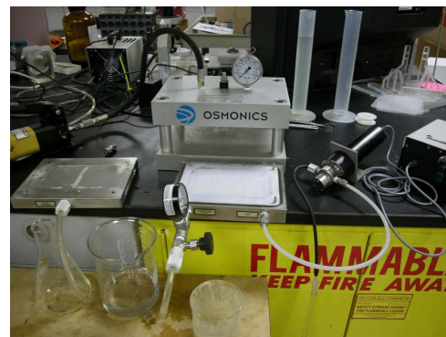
Figure 1. An ultrafiltration membrane (white piece of sheet near the center of the photo) is mounted in a GE Sepa CF II filtration test system for testing.
