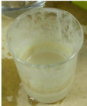
Figure 3. Microwave cooked baking yeast solution used as a foulant in the experiment.
