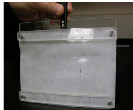
Figure 8. The membrane cleaned and to be tested with the GE Sepa CF II filtration test system in Figs. 1 and 2.
