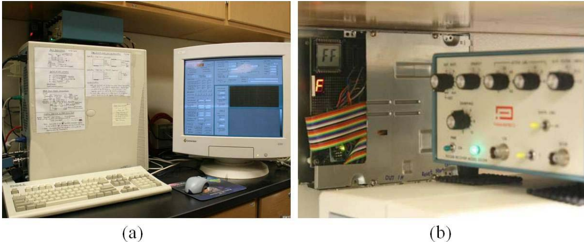
Figure 10. Motor controlling system. (a) shows the software for controlling motor movement and sending triggers for HFR system. (b) shows the counter for counting trigger number.
