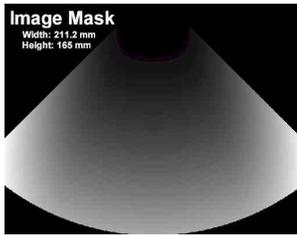
**Figure 3.** Image mask with both angular and axial amplitude compensations. The mask is normalized to the brightest point.
