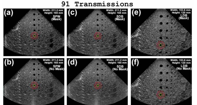
**Figure 6.** Effects of masks on images reconstructed with the HFR imaging method with 91 transmissions. 50 dB log compression has been applied..
