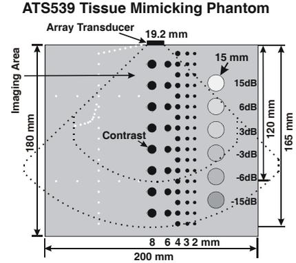
**Figure 4.** A cross-section of an ATS539 tissue-mimicking phantom showing the imaging areas of 120 mm and 165 mm depths with  $\pm 45$  degree field of view for the experiments. (Modified from Fig. 2 of the 2011 IEEE IUS diverging beam paper [5].)
