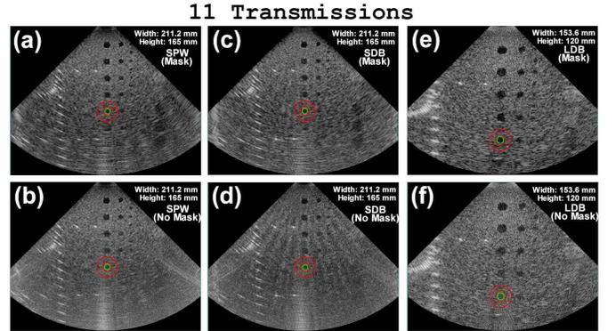
**Figure 5.** Effects of masks on images reconstructed with the HFR imaging method with 11 transmissions. 50 dB log compression has been applied.
