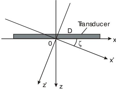
**Figure 1.** Rotation of coordinates from  $(x, z)$  to  $(x', z')$  by a steering angle  $\zeta$ .
