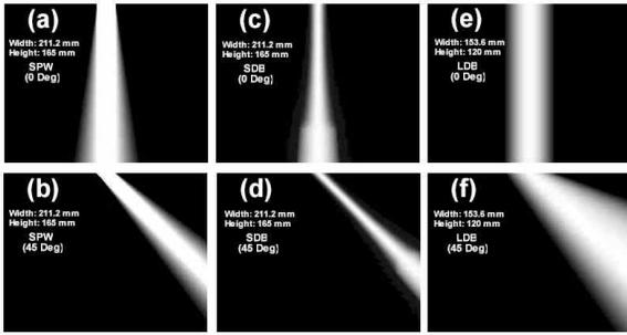
**Figure 2.** Strip masks for SPW, SDB (9 degree divergence), and LDB at both 0 (top row) and 45 degrees (bottom row). The masks are normalized to the brightest point.
