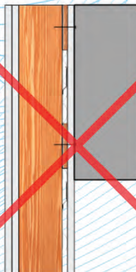
Base Wall + Cabinets & Plywood Backing
